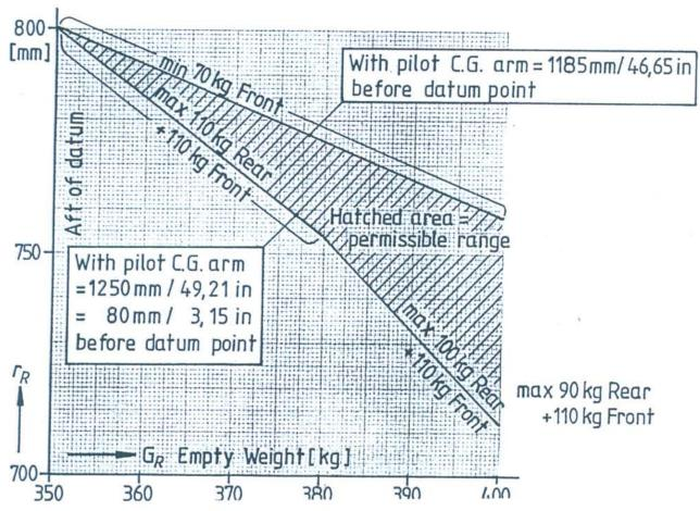
The CG should be recalculated after repair, repainting or installation of additional equipment, but not later than 4 years after the last weighing.
